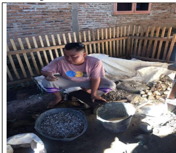
Figure 1. Process of crushing containing rock gold at home public.
