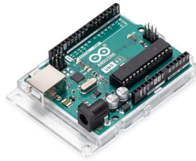
Figure 4. Arduino Uno R3 [10]
