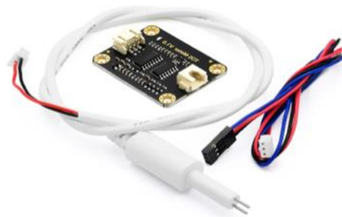
Figure 5. Analog TDS sensor module water solubility conductivity SEN0244
